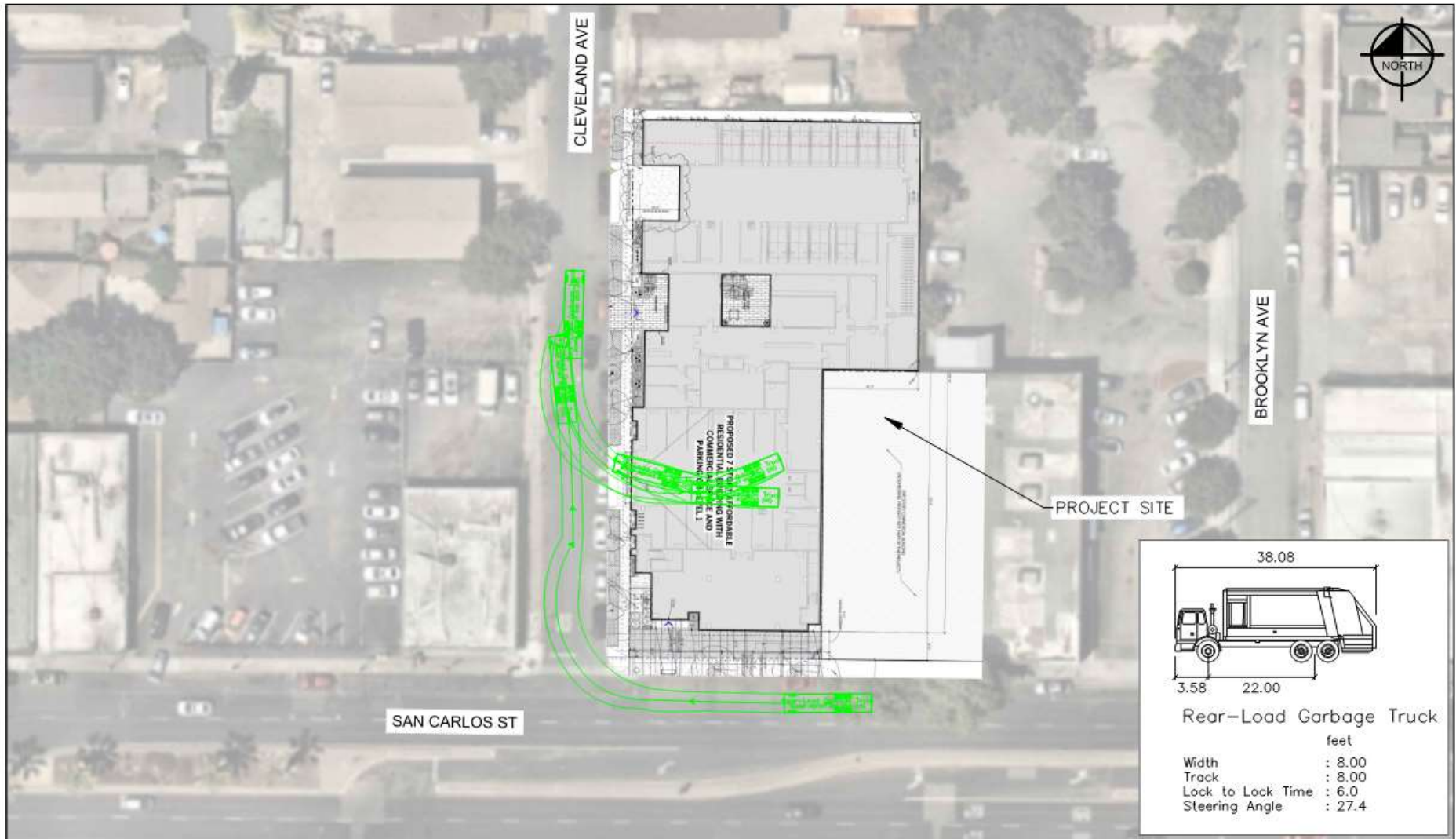
Figure 16: Garbage Truck Access
