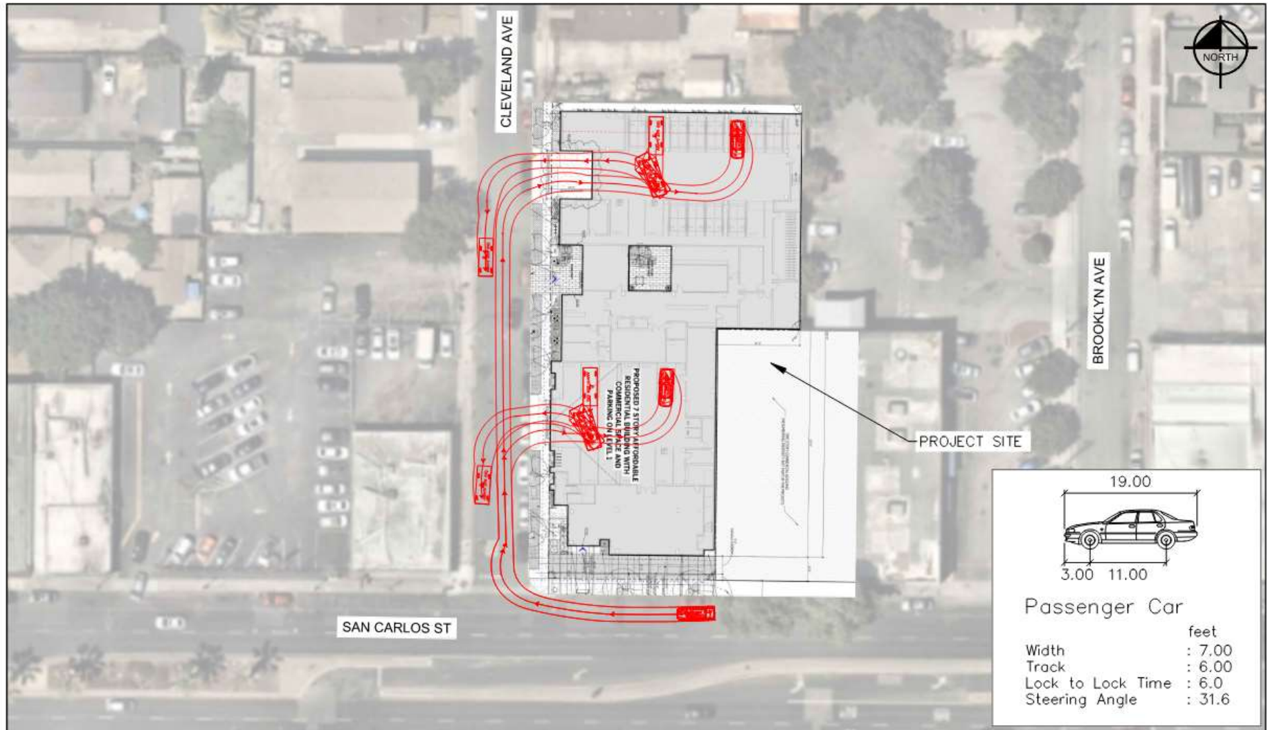
Figure 15: Passenger Vehicle Access
