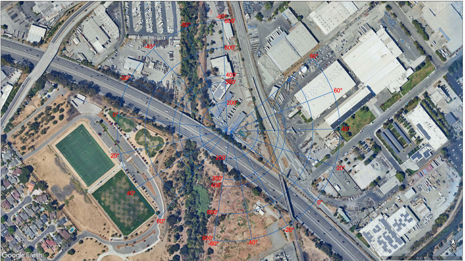
Figure 4. Site satellite photo overlay of distances and angles from proposed digital billboard site, corresponding to calculated illuminance figures in fc provided in Table 1.
