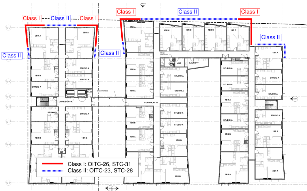
Figure 6: Second through Fifth floor glazing assemblies acoustical rating recommendations to satisfy CCR Title 24 requirements. Windows of units not labeled are not required to possess acoustical rating.
