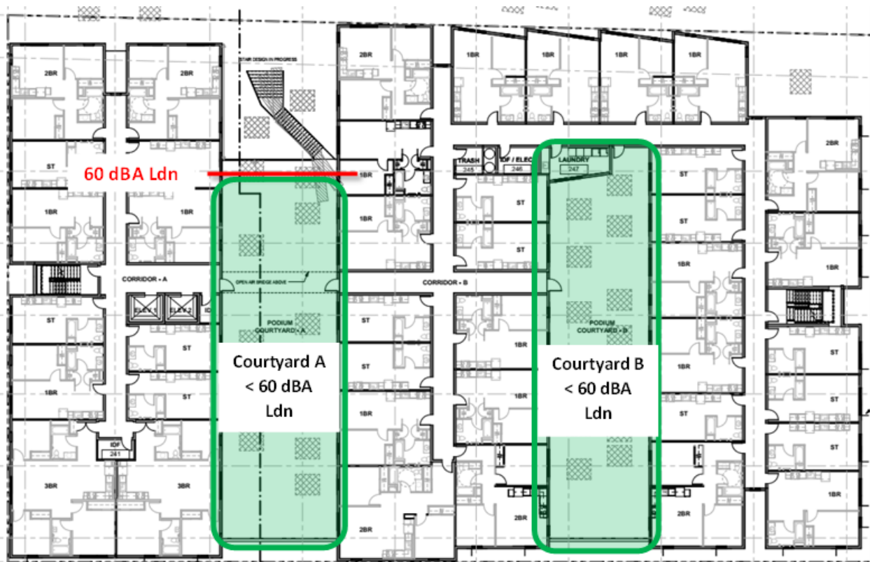
Figure 7: Floor plan showing second floor exterior courtyards. Green zones indicate areas of the courtyards calculated to have an Ldn of less than 60 dBA based on shielding calculations. A contour line for 60 dBA Ldn is shown at the north end of Courtyard A, denoting parts of the courtyard that are above the City criteria for outdoor spaces.
