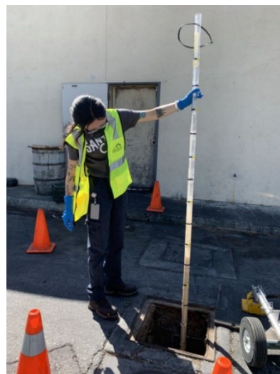
FIGURE 27. GREASE INTERCEPTOR SAMPLING
