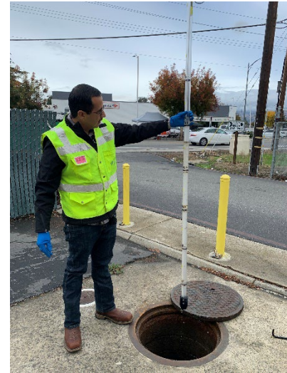
FIGURE 27. GREASE INTERCEPTOR SAMPLING
