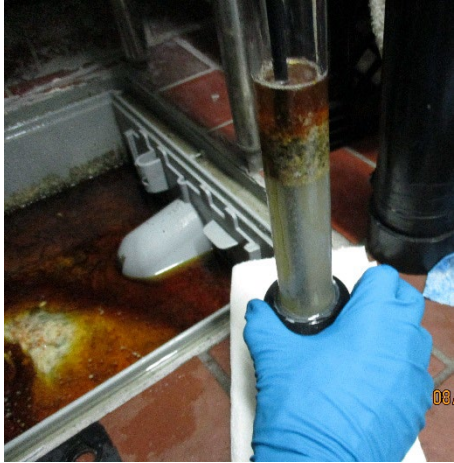
FIGURE 23. ENVIRONMENTAL INSPECTOR TAKING A CORE SAMPLE FROM A GREASE TRAP
