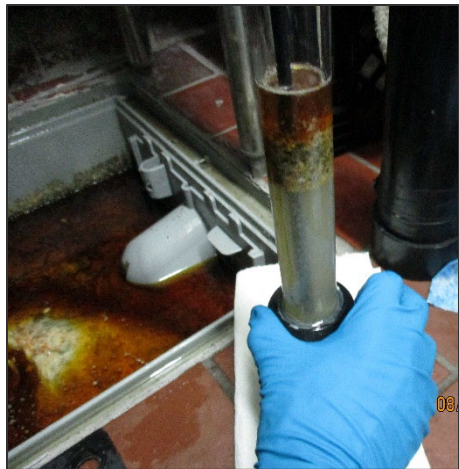
FIGURE 29. ENVIRONMENTAL INSPECTOR TAKING A CORE SAMPLE FROM A GREASE TRAP
